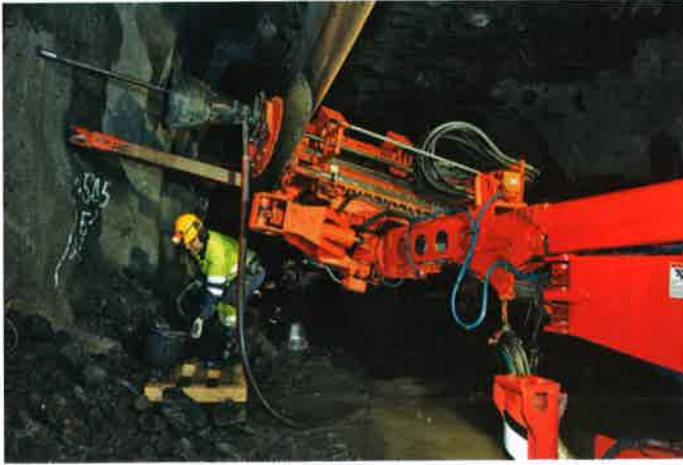
Sandvik DL430-C being used on this occasion for sludge drilling and sampling to define the orebody in an area where only limited core drilling has been undertaken. Picture by Eija Hiltunen
