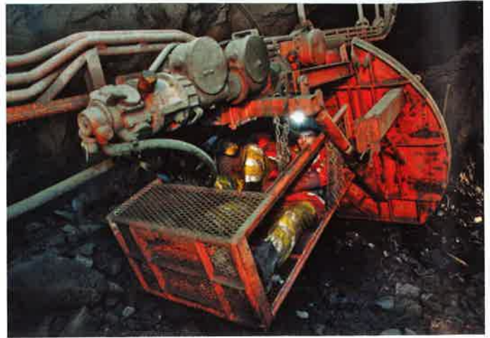
Alimak raise miner in action. Picture by Eija Hiltunen
